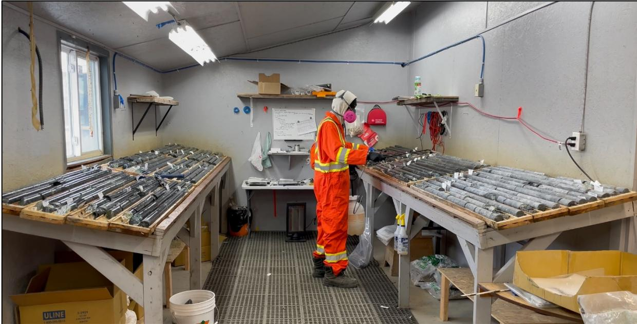
Figure 2-3. Core processing room with worker wearing personal protective equipment (PPE) during the logging and sampling process as part of the Company’s procedures and protocols.
