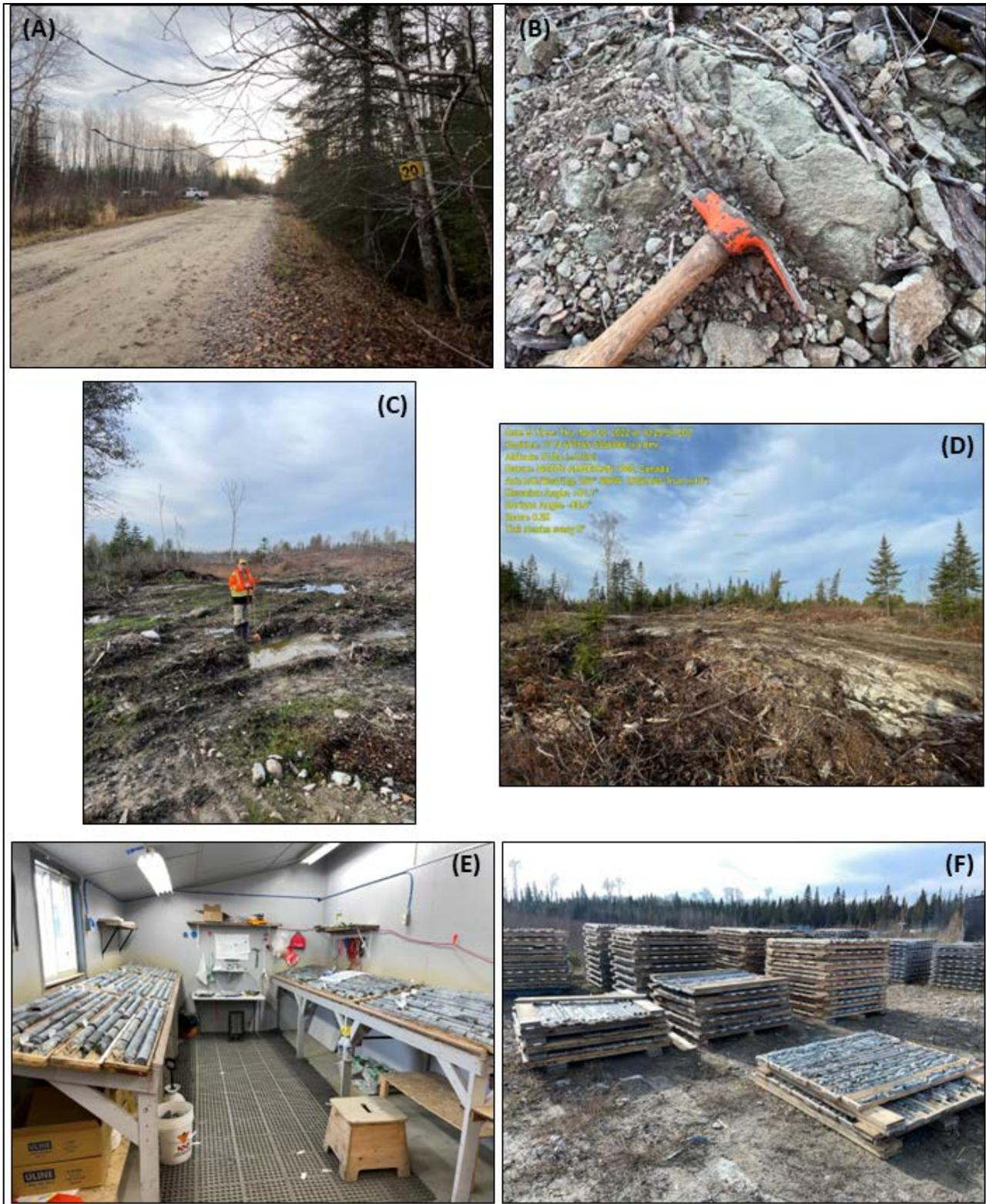
Figure 2-2. Selection of photos taken during the Personal Inspection of the CarLang Nickel Property by Co-Author John Siriunas. (A) All weather access road (Stringer's Road), to the Property; (B) Exposed, heavily altered, ultramafic rocks on the Property; (C) Co-Author John Siriunas standing at marked diamond drill collar; (D) Typical exposure and physiography at the Property; (E) Core logging facility at Redstone Mill Facility; (F) Cross-piled core storage at the Redstone Mill Facility.
