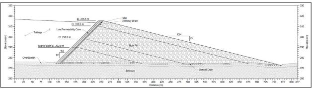
Figure 18-2: Typical dam cross-section.
