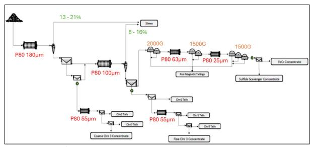
Figure 13-5: CNC Crawford Open Circuit Test Flowsheet.
