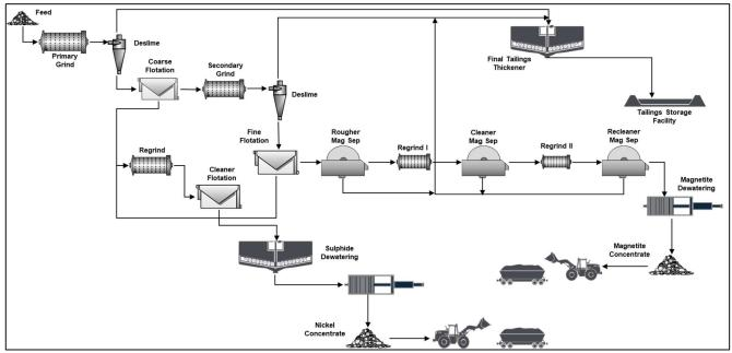
Figure 17-1: Schematic of process flowsheet.
