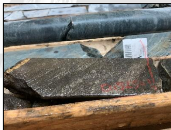
W4- Hole EV21-01§ Pentlandite sample Grading 17.6% Ni
