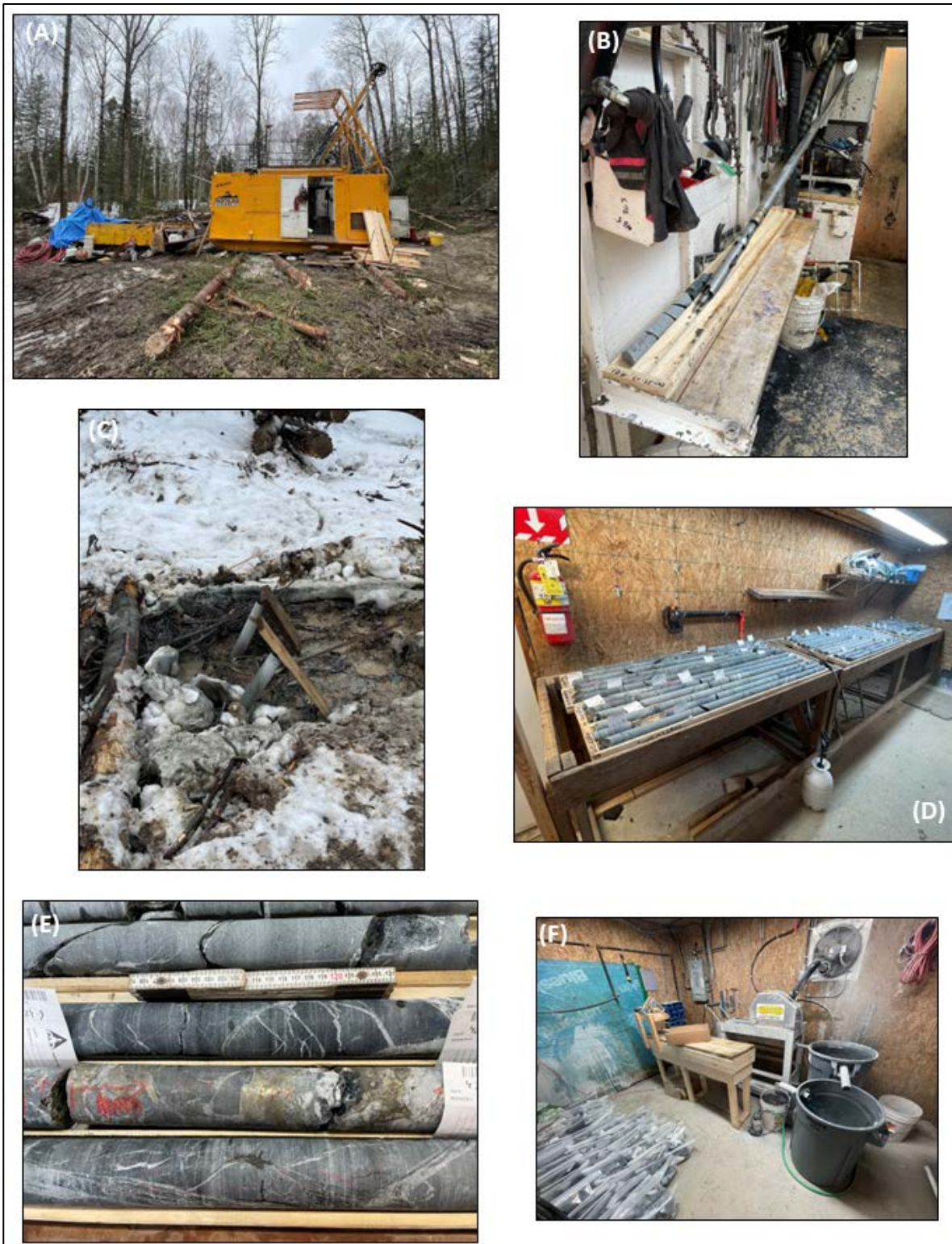
Figure 2-2. Selection of photos taken during the Personal Inspection of the Property by Co-Author John Siriunas. (A) Diamond drilling at the site of EV23-03; (B) Core and core barrel ready for the extraction of drill core from the most recent “run” in hole EV23-03; (C) Casing at holes EV23-01 and EV-23-02 prior to capping and flagging; (D) Drill core laid out for logging and marked for sampling; (E) Drill core with massive sulphide sections in the vicinity of 425 m, EV23-02; (F) Core cutting saw and samples prepped for transport to ALS laboratory.
